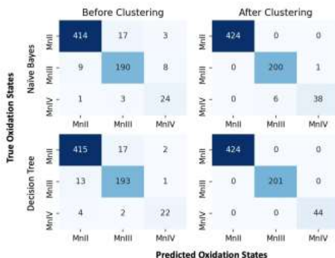
Fig. 3. The confusion matrix of GNB (top) and DT (bottom) prediction models before (left) and after (right) k-mean clustering.
