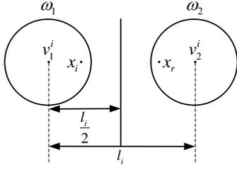
**Fig. 3** Clustering result of FCM for pixel  $x_i$  and pixel  $x_r$ , pixel  $x_i$  belongs to cluster  $\omega_1$  and pixel  $x_r$  belongs to cluster  $\omega_2$
