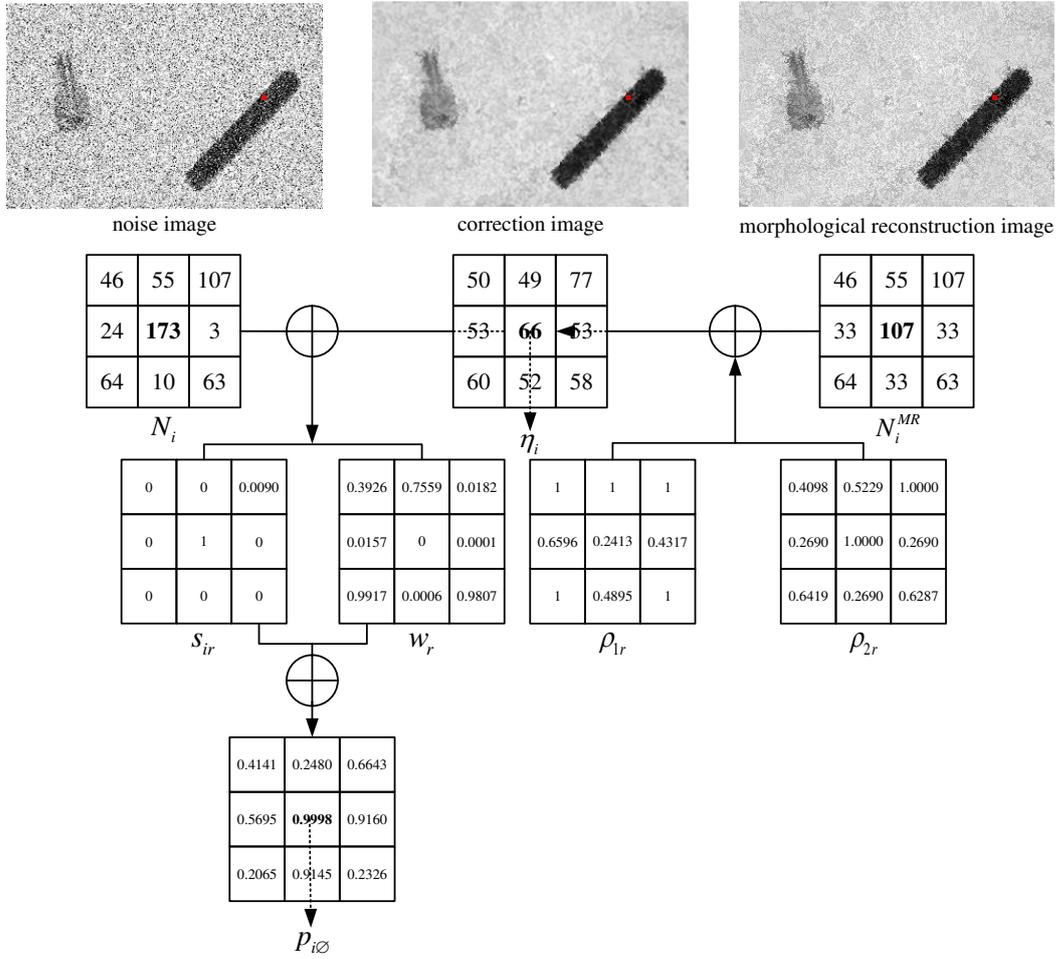
**Fig. 4** The process of calculating the noise probability  $p_{i0}$
