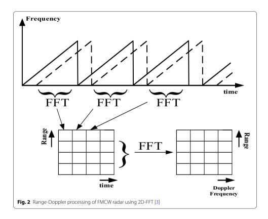
processed in both directions using 2-D FFT. The first FFT is used to extract the target range by calculating the Fourier in the range direction only. The second one is used in the azimuth direction to extract the Doppler component, as shown in Fig. (2).
