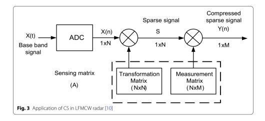
If the radar signal samples with dimension, N, are transformed into under-sampled signals or measurements, M, with a linear operator where the measurement vector, y, is given by:
