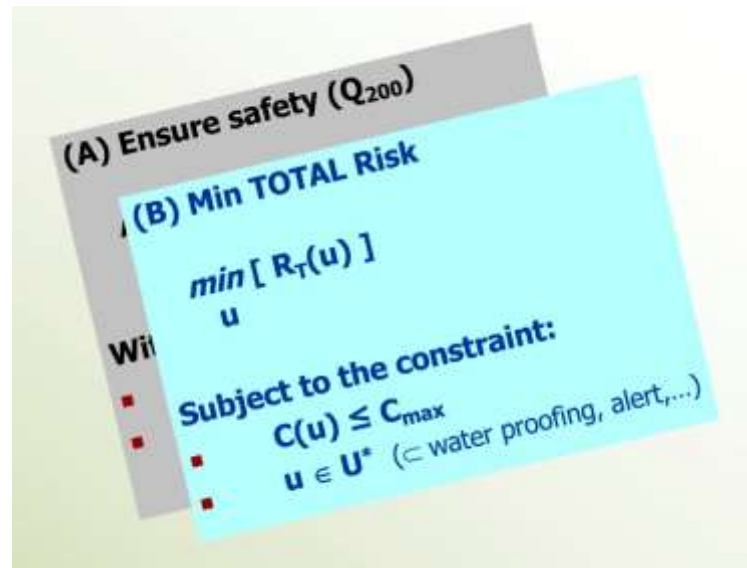
Figure 3. An evolved paradigm centered on the total risk R_T including the residual risk ( R_R ), and a broader spectrum U^* of possible interventions, under a maximum expenditure constraint C_{max} . A further evolution may recognize a multidimensional nature of the risk (e.g., tangible, intangible).
