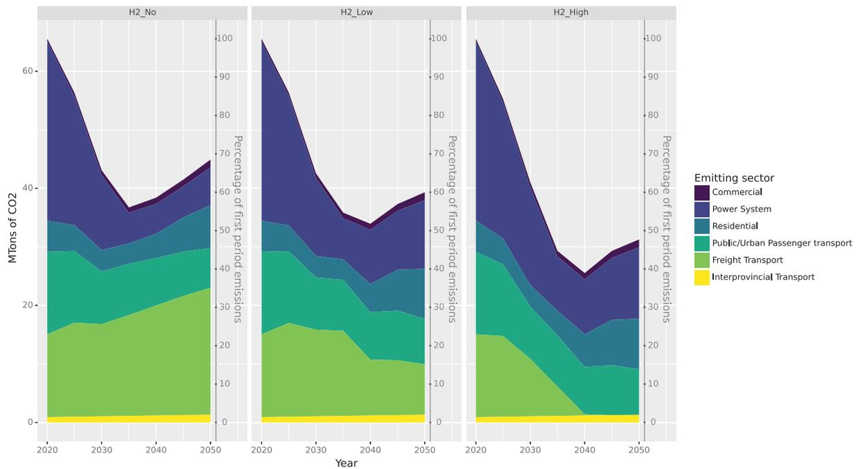
Fig. 5. Total CO<sub>2</sub> emissions for all hydrogen scenarios without emission constraints.
