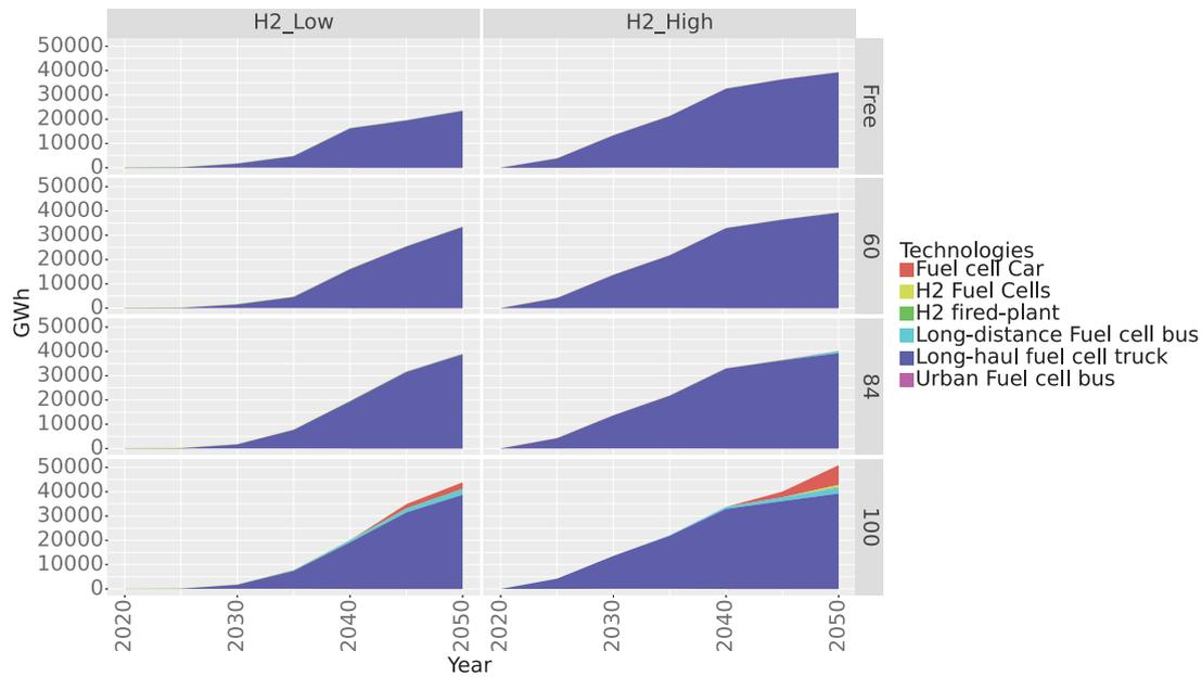
Fig. 7. Hydrogen consumption per vehicle type for all hydrogen and emission scenarios.
