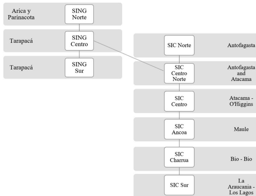
Fig. 2. Diagram of transmission lines and representative nodes from Babonneau et al. (2021). White boxes represent the nodes that simplify the national electricity system, while the names in the gray rectangles represent the approximate geographic location in Chile's regions covered in this study.
