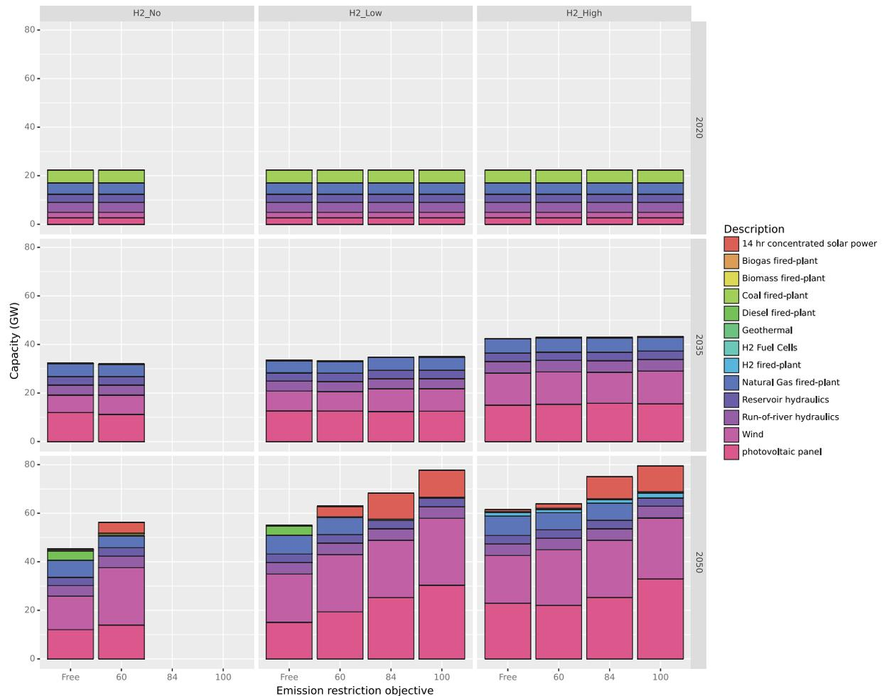
Fig. 10. Global installed capacity of power sector by year, scenario and emission restriction objective.
